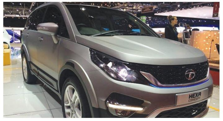
Tata Motors, the home-grown automajor, has unveiled a new SUV concept - the Hexa at the ongoing 2015 Geneva Motor Show. The concept is based on the Aria platform and features a 2.2-litre, fourcylinder, VARICOR diesel unit that is good for 154bhp and 400Nm. The car is 4764mm long, 1895mm wide, 1780mm tall and has a
